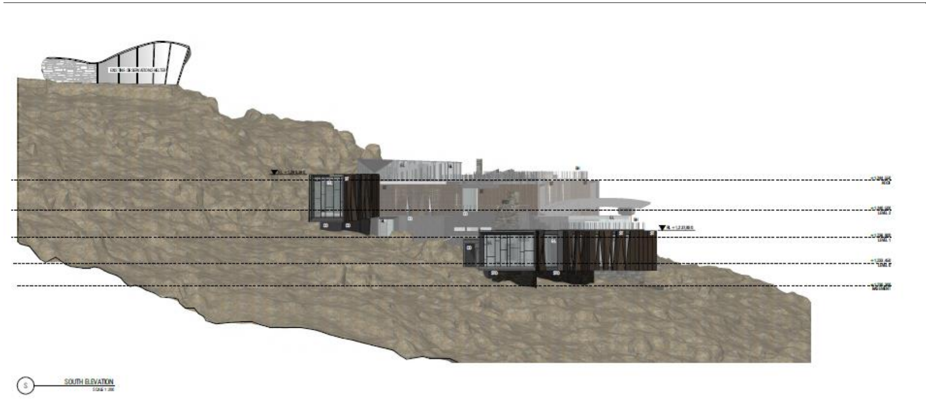
Figure 2: Building design from perspective of southern elevation, showing north and south sections of the building, the adjoining enclosed glass walkway, and the proposed obstructions on eastern face windows that may have posed a reflective risk
