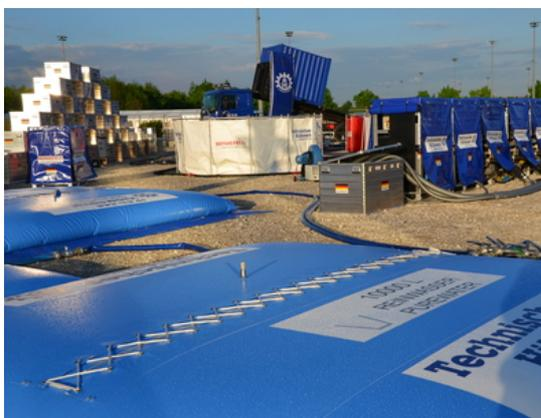
Fig. 44: Mobile water treatment plant (THW, 2016)
