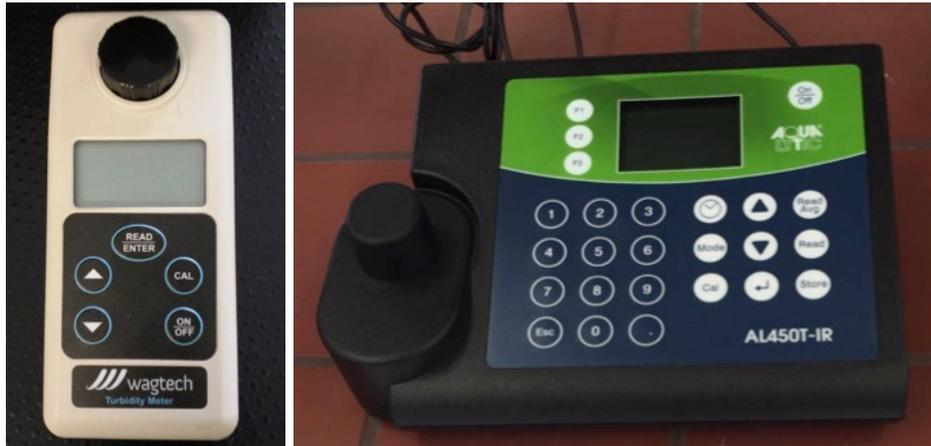
Fig. 35: Portable Wagtech Turbidity Meter used for on-site testing (left), Aqualytic Turbidity meter used for laboratory testing (right)
