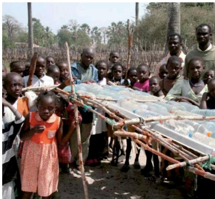
Fig. 72: Solar disinfection with PET-bottles in Senegal (SODIS, 2016)
