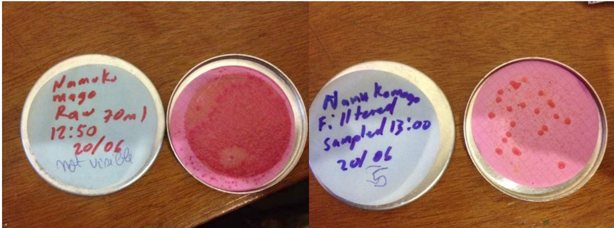
Fig. 57: Plate counts (total coliforms) of Namukomago (20/06/2016), raw-water (right), filtered water (left)
