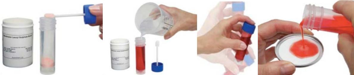
Fig. 25: Preparation of the liquid nutrient media (MLSB) and the nutrient pads, schematic sketch (Wagtech, 2013)
