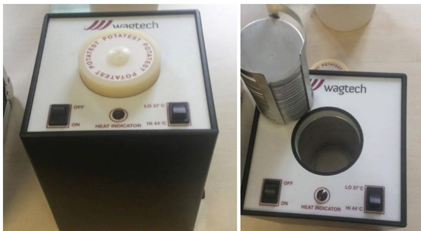
Fig. 26: Wagtech Potatest mobile Incubator, closed (left), opened with petri dishes (right)
