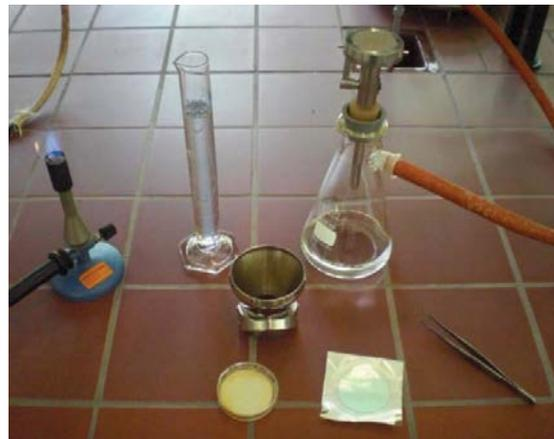
Fig. 18: Needed materials and devices for the membrane filtration method (DANY, 2011)
