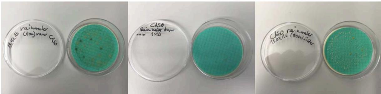
Fig. 63: Plate counts (HPC) of rainwater (barrel), laboratory testing
