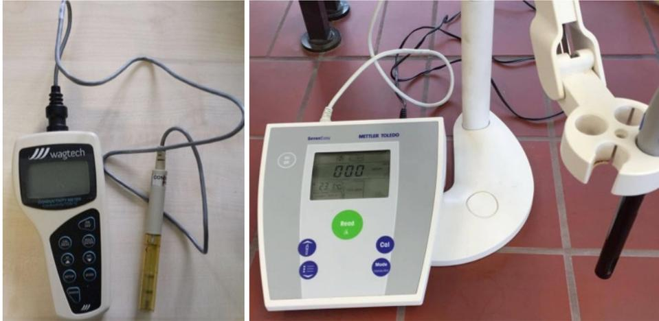
Fig. 31: Portable Wagtech turbidity meter used for on-site testing (left), Mettler Toledo Conductivity meter with measuring electrode used for laboratory testing (right)
