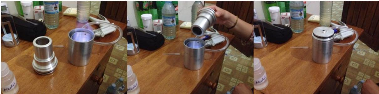
Fig. 27: Process of disinfecting the mobile membrane filter unit: burning alcohol within the containment vessel (left), putting in the separated MTU (middle), disinfection through anaerobic vapour (right)
