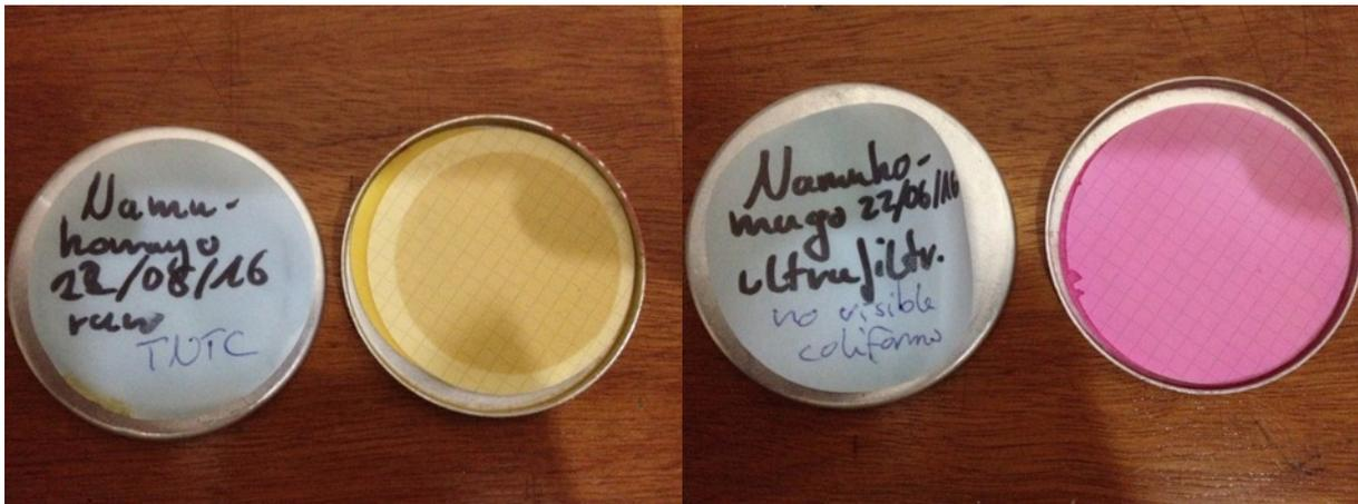
Fig. 55: Plate counts (total coliforms) of Namukomago (22/06/2016), raw-water (left), filtered water (right)
