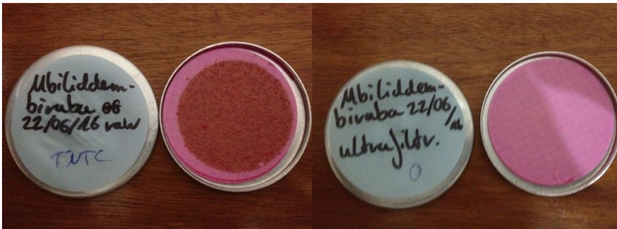
Fig. 54: Plate counts (total coliforms) of Mbiliddembiraba (22/06/2016), raw-water (left), filtrated water (right)
