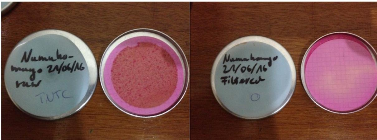
Fig. 53: Plate counts (total coliforms) of Namukomago (21/06/2016), raw-water (left), filtrated water right)
