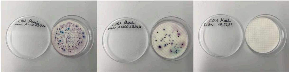
Fig. 62: Plate counts (E.Coli and coliforms) of river water (Moselle), laboratory testing
