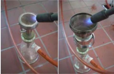
Fig. 19: Sterilisation of the porous metal plate (left) and funnel attachment (right) (DANY, 2011)
