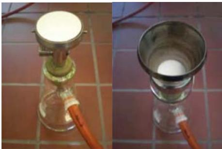
Fig. 20: Membrane filter on-top of porous metal plate (left), funnel attachment placed at the device (right) (DANY, 2011)
