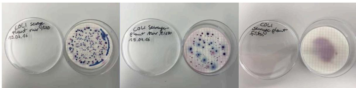
Fig. 61: Plate counts (E.coli and coliforms) of sewage plant effluents, laboratory testing
