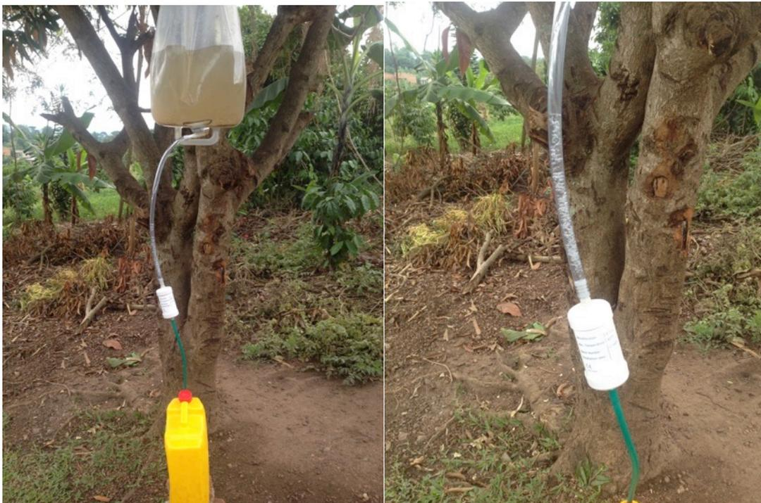
Fig. 52: Filtration of raw-water in Namukomago, with detail (right)
