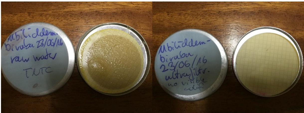
Fig. 56: Plate counts (total coliforms) of Mbiliddembiraba (23/06/2016), raw-water (left), filtered water (right)
