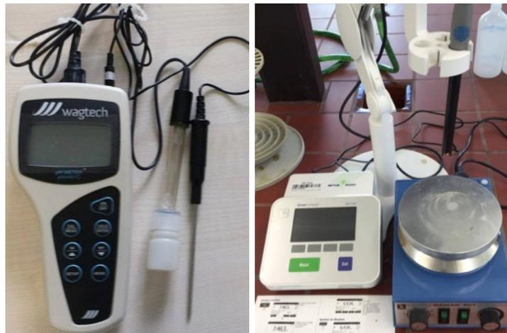
Fig. 30: Portable Wagtech pH meter for on-site testing (left), Mettler Toledo pH meter with measuring electrode and magnetic stirrer for laboratory testing (right)
