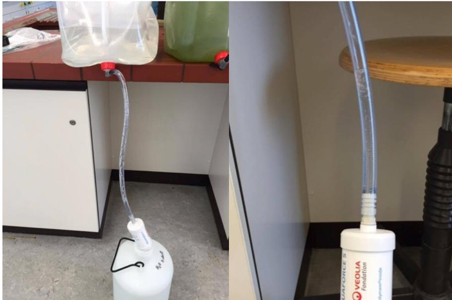
Fig. 58: Filtration of raw-water samples in the laboratory, with detail (right)
