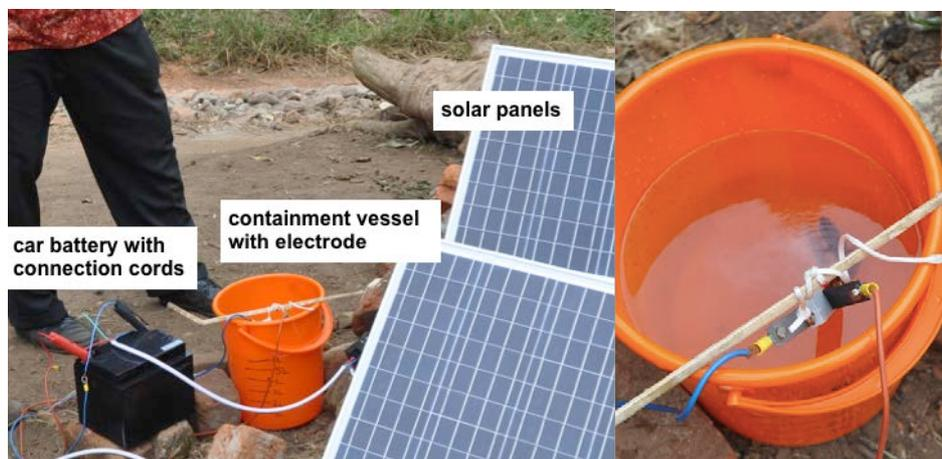
Fig. 41: Chlorination system, on-site prototype with solar panels to recharge batteries (left), electrodes with temporary fixing, detail (right), edited
