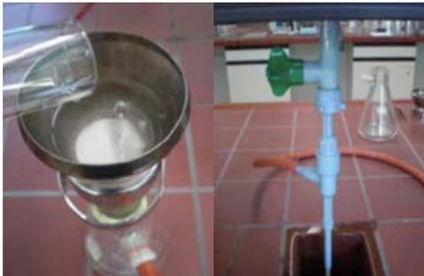
Fig. 21: Addition of water sample (left), water jet pump (right) (DANY, 2011)
