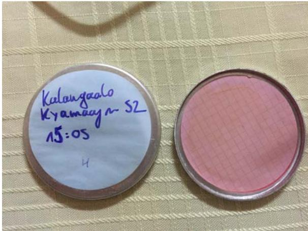
Fig. 38: Plate Count (total coliforms) of Kyamagemule, 12.06.2016, 4 cfu/200 ml
