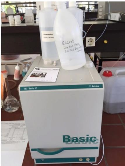
Fig. 32: Ion chromatograph, exterior
