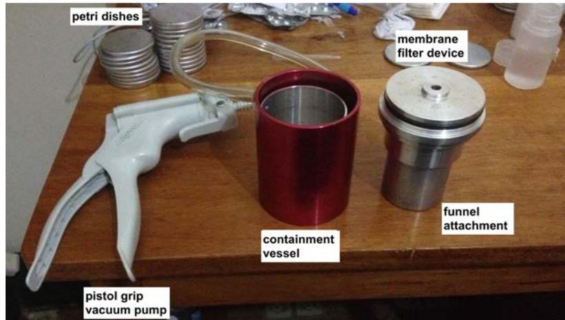
Fig. 23: Mobile membrane filtration unit (MFU) with pistol grip vacuum pump (left), edited
