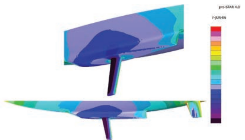
CFD work for Athos, heel 20°, drift 3°
