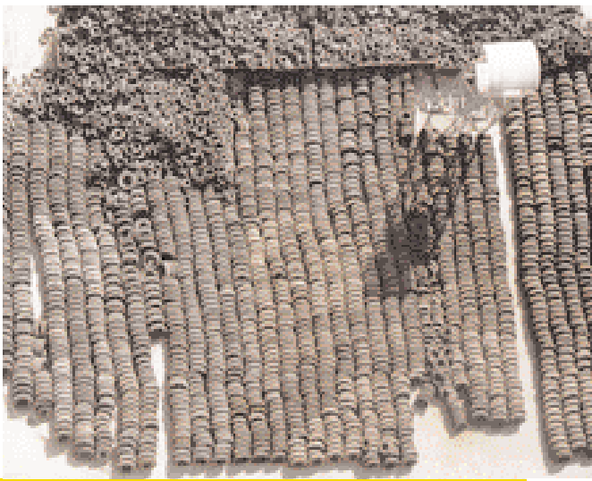
CZECH REPUBLIC | Cement | Stock of tires used as an alternative energy source at the Cizkovice cement plant
