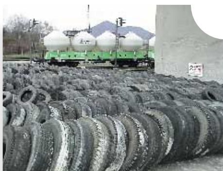
Czech Republic - Utilisation of used car tyres as a source of energy at the Cizkovice cement plant
