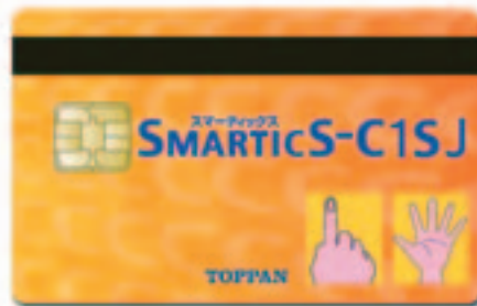
An IC cash card capable of authenticating the palm and finger veins of the “cardholder”
