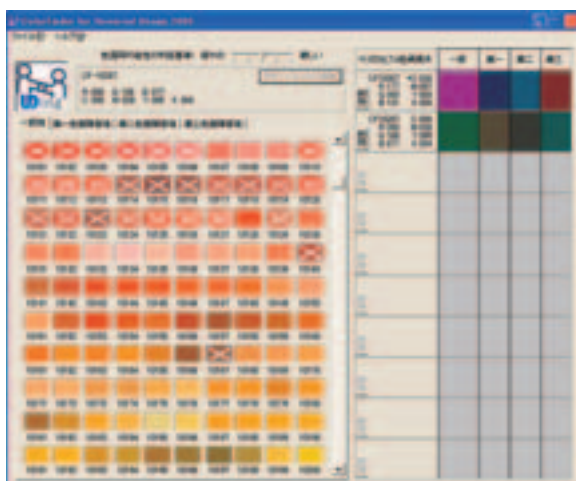
The CFUD tool finds colors that can be easily distinguished by people with defects in color perception.
