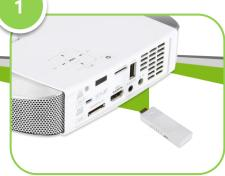
Connect transmitter to video source devices.
