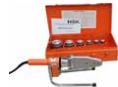
Heizelemente socket welders
