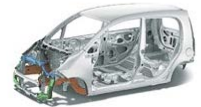
Advanced Compatibility Engineering (ACE) body structure
