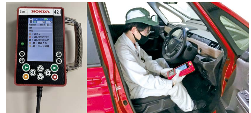
Inspection using the LET system
