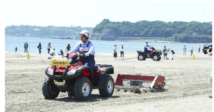
Honda Beach Cleaner that can dig up and collect trash in the sand.
