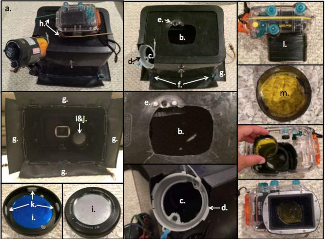
Figure 26. Configuration of ‘dark box’ setup for the fluorescence census technique. Letters in the figure correspond to the methodology text.
