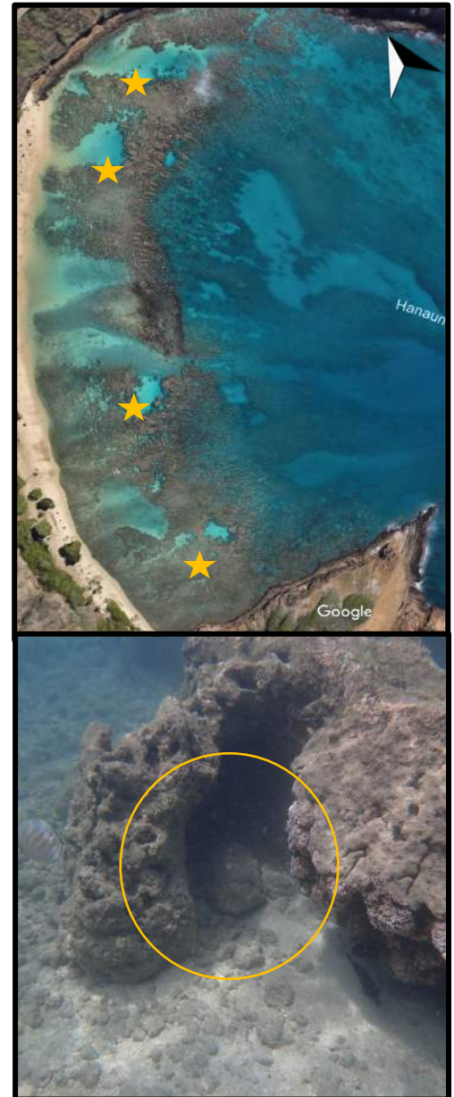
Figure 40. Location of temperature loggers within the inner reef flat of the Hanauma Bay Nature Preserve (top photo). Example of concrete "rock" with temperature logger (bottom photo).
