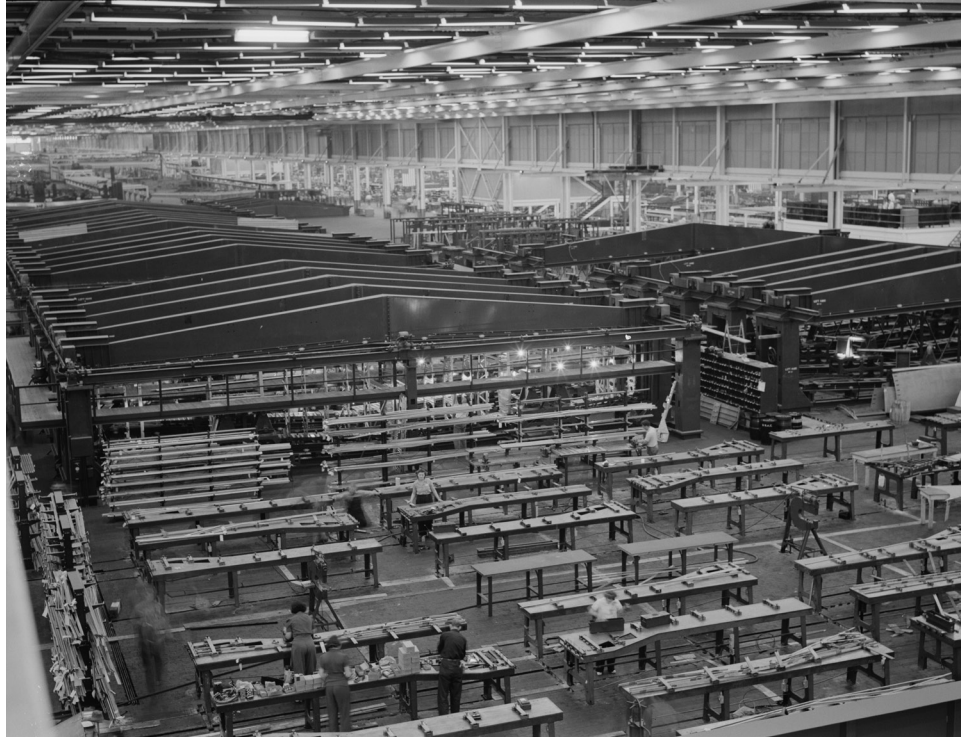
Ford Motor Company bomber factory at Willow Run, Michigan, in 1942. This was the world's largest one-story war production plant. Fixtures in the background held bomber wings during assembly. Note the women workers. No one could say that crime was caused by unemployment during the 1940s, because jobs were widely available.
