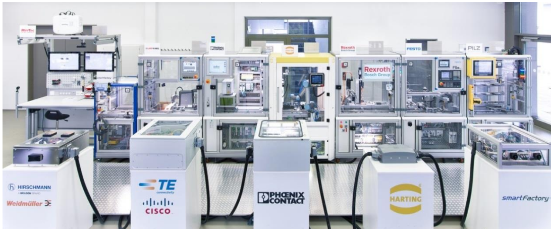
Figure 24: Modular production system in the SmartFactory
