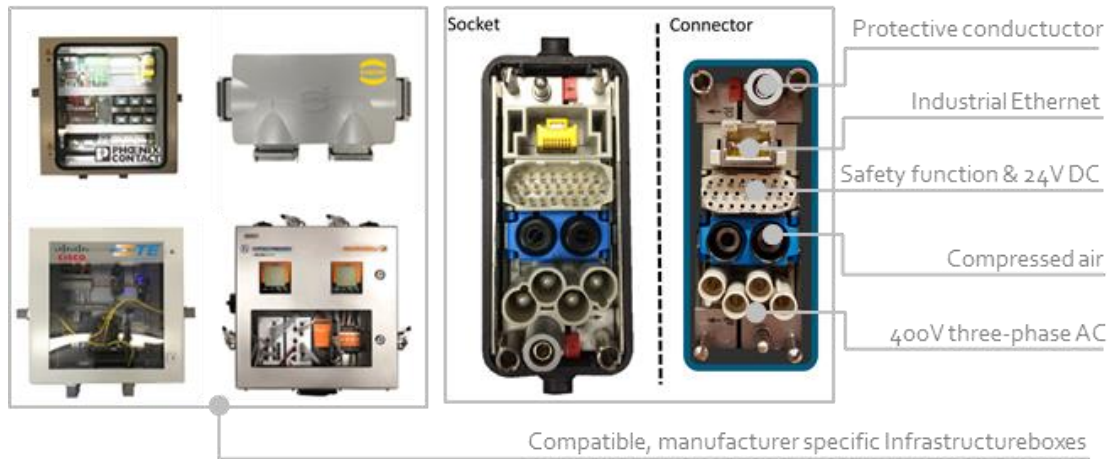
Figure 29: Modular Infrastructure Box (left) and Socket/Connector (right)
