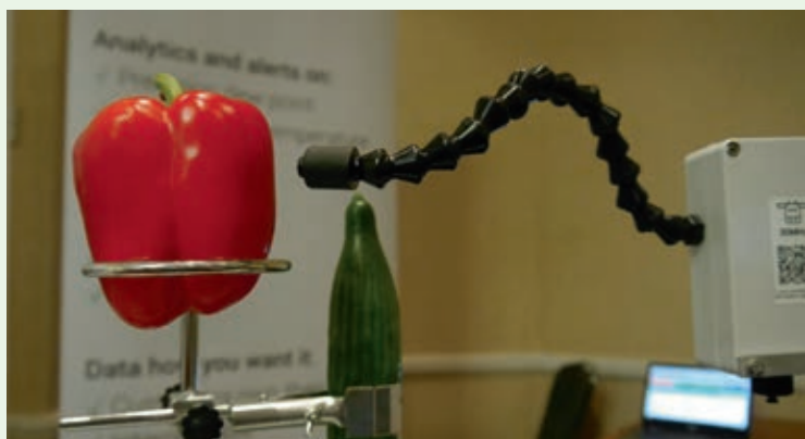
The 30MHz sensor for monitoring the surface temperature of fruits or leaves.
