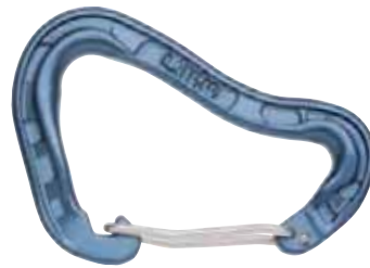
CATCH CE UIAA WIRE 33 g slate 663 Extremely light and shapely karabiner. A special hot forging technic allows the best use of the material and a fine surface finish. The double T construction guarantees the highest breaking strain for the minimal weight. The large radius ensures the best possible treatment of the rope. 71807
