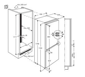
Sliding door fixing (HxWxD) in mm 1780 x 560 x 550
