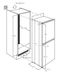
Door-on-door fixing (HxWxD) in mm1780  $\times$  560  $\times$  550
