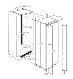
Sliding door fixing (HxWxD) in mm 1780 x 560 x 550
