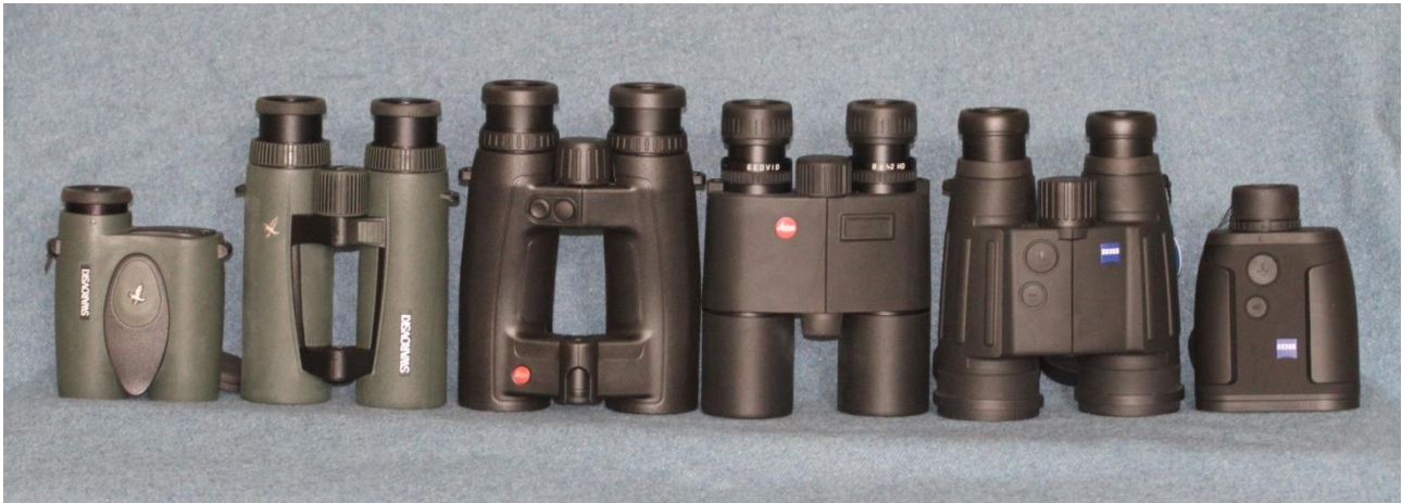
Picture 18. Different rangefinders to compare with the Leica Geovid 8x42 BD: from left to right: Swarovski Laserguide 8x30, Swarovski EL Range 8x42, Leica Geovid 8x42 BD, Leica Geovid 8x42HD, Zeiss 8x45 RF, Zeiss RPF 8x26
