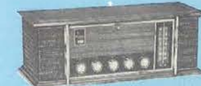
ARVIN AUTOMATIC AM/FM MULTIPLEX STEREO RADIO Automatic multiplex circuits for FM stereo reception. 9 tubes plus rectifier and 5 diodes with push-pull circuit and feedback tone control. Two acoustically balanced 5" Velvet Voice speakers. Lighted slide rule dial tuning, full range tone control and stereo-balance control. Line cord FM antenna, ferrite rod AM antenna plus external FM antenna terminals. Color: Walnut Hardwood. 7 1/2" x 18 1/2" x 6 1/4". Shpg. wt., 17 lbs. 33R68 S7347 $99.95
