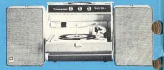
GENERAL ELECTRIC STEREO PHONOGRAPH—TRILINE "300" Vinyl heat pressure laminated steel case with push latch. 4-speed automatic flip-down changer. Four 6 1/2-inch Dynapower speakers that can be detached and separated, up to 25 feet with the included permanent extension cords. 45 RPM spindle included. One triode section and one power pentode amplifier in each stereo channel. Loudness, channel balance and continuous variable tone controls. Tape recorder can be plugged into output jack. Colors: Driftwood Brown, or Antelope White. 14" x 24 1/2" x 9". Shpg. wt., 37 lbs. *RP2153 S9795 $129.95
