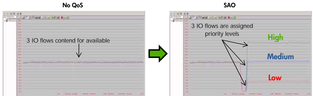
Figure 2: Performance impact of SAO and QoS. With SAO enabled, IOs are categorized into priority levels.
