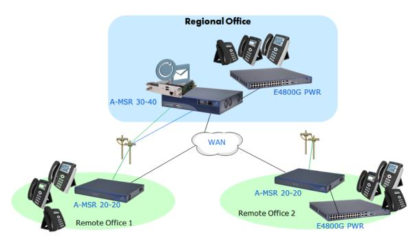
An example of VCX Connect 200 and VCX Connect MIM in a VCX Multi Region configuration is shown below.
