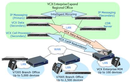
Take advantage of the VCX architecture to include HQ and many Branches. Combine HQ plus a large distributed network into a single entity that provides the look and feel of a single system to users with Global Directory and Global Voice Mail services. An example of VCX V7000 Expand in a Multi Region configuration is shown below, with a VCX V7000 Classic for the HQ and a VCX V7000 Expand for all the Branch Offices.
