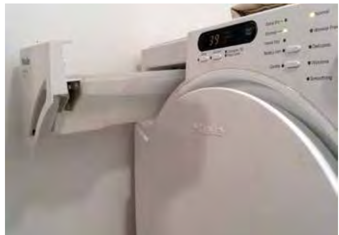
Ventless appliances reduce the ventilation load, however, this clothes drier dumps a considerable amount of heat back into the room. Passivhaus eco-buildings with ventless appliances will roast inhabitants unless companion mechanical cooling is provided. Non-potable water removed from clothing can be collected in the tank and used for watering plants.
