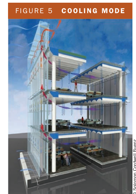
In cooling mode (designed to operate 50 days per year), a ducted underfloor air system provides ventilation air and supplements the radiant ceiling cooling system on design days.
