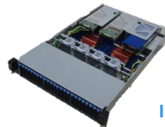
R280-F38 / F3C / F28 / F2G / F2O (MB=MD90-FS0) 2 x FHHL & 6 x FHFL & 1 x Universal I/O Support 3 GPGPUs
