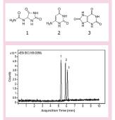
Peaks: 1. Allantoin 159.0513 m/z [M+H]<sup>+</sup> 2. 6-aminouracil 128.0455 m/z [M+H]<sup>+</sup> 3. Uric acid 169.0356 m/z [M+H]+
