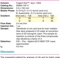
metabolites is simple and doesn't require mobile phase additives or pre-column derivatization. The peaks are symmetrical and the MS signal is not diminished, as is the case when ammonium for-mate or acetate is used as a mobile phase additive. The analyzed metabolites are signature end products for UA degradation in the presence of oxidants and can therefore be used as biomarkers for different disease states.
