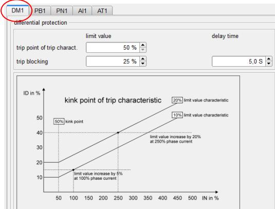
For adjustment of differential protection settings the DM1 module has to be enabled via tab „basic settings“. „Watchdog“ alarm will be tripped if the module is enabled but not connected to bus.
