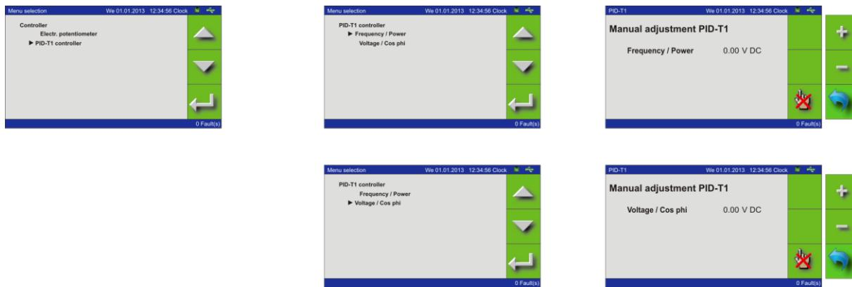
The two available PID-T1 controllers have to be assigned to an analog output. Setting of the adjustment range is solely done via the parameter software.
