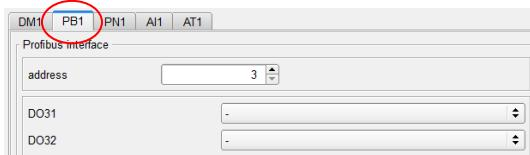
For adjustment of profibus coupling settings the PB1 module has to be enabled via tab „basic settings“. „Watchdog“ alarm will be tripped if the module is enabled but not connected to bus.
