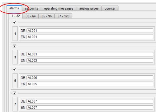
128 alarm messages are available. The alarm texts can be input in the corresponding fields. In case of an inactive alarm the field is shown grayed. The behaviour of the single alarms is set within the PLC.
