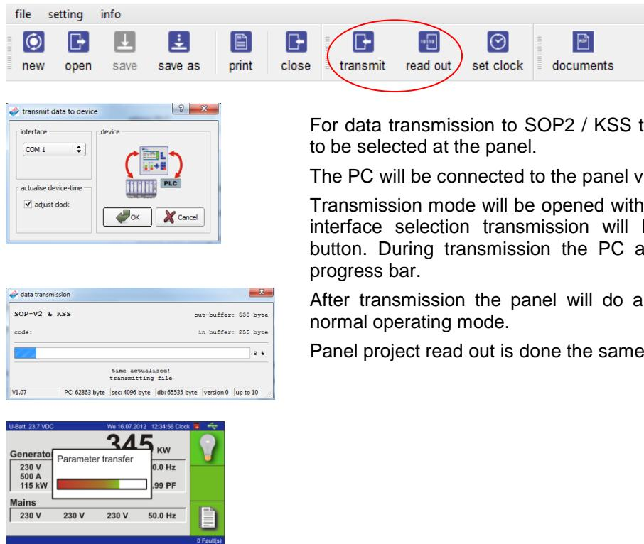
For data transmission to SOP2 / KSS the operating mode „0“ has to be selected at the panel.
