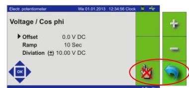
Two electronic potentiometers are available. The potentiometers have to be assigned to an analog output to be able to do adjustments via panel. The internal signals of the pulse controller influence the adjustment of the electr. potentiometers. Setting of the adjustment range of the electr. potentiometer is solely done via SOP 2. However the values can be read and displayed with the configuration software Device Management 2.
