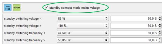
This function has to be activated. If this function should not be enabled permanently it is possible to lock it via a digital output parameterized accordingly.
