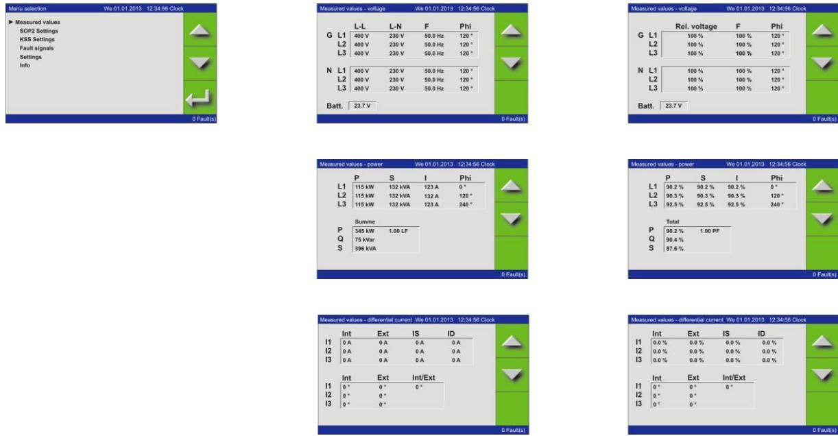
The Operator Panel displays six different screens for measured values:
