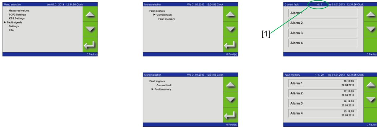
All pending error messages are listed in the screen „Current fault“. If there are more than 4 alarms pending, it is possible to browse them by blocks. The upper status bar [1] displays the total number of alarm messages pending, and visualizes the block just browsed.
