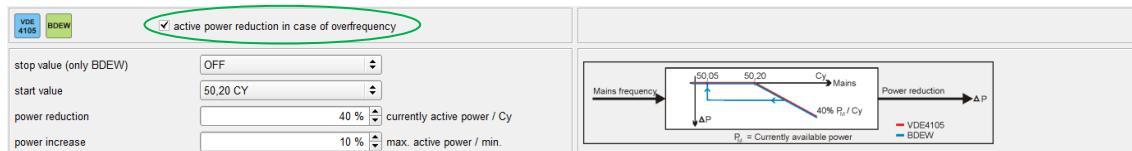
This function has to be enabled. In the operation, there are differences between VDE4105 and BDEW.
