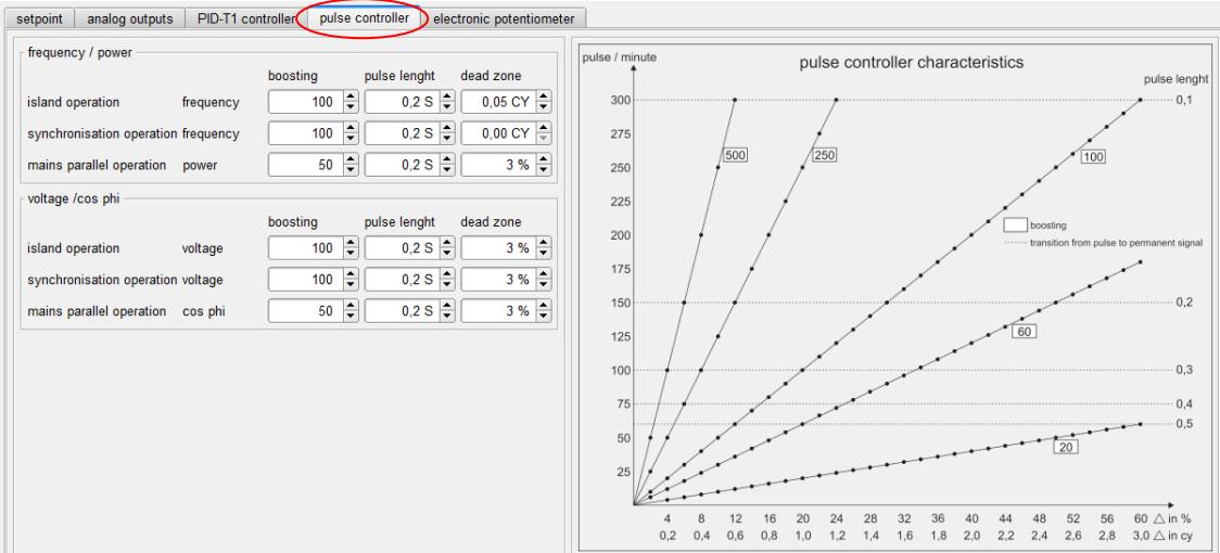
Settings for controller characteristics. Each operation condition has its individual settings. Controller settings affect the pulse controller (output via digital outputs), as well as the electr. potentiometer adjustments.
