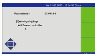
If there is no PC available all parameters can also be adjusted directly at the SOP2. The input is protected by a PIN.
