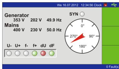
The SYN screen can **NOT** be selected with the arrow keys. During active synchronization the screen is automatically displayed, and as well automatically faded out after synchronization.
