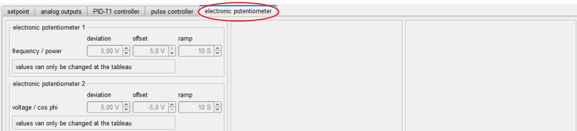
Input of electronic potentiometer values is only possible via panel. When visualizing the parameter data only the values input via panel are displayed.
