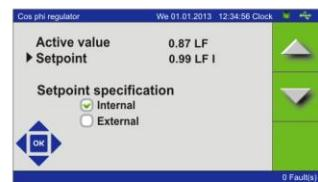
Setpoints can be set for two different regulators. For the setpoint specification selection is possible between the setpoint adjusted at the panel (internal) or the analog value (external). When not activated via parameterization the menus for these regulators are greyed out and cannot be selected.
