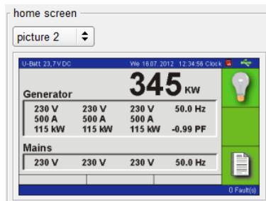
All measured values available in the KSS can be displayed with the SOP2. For further screens please go to the parameter "measured values".
