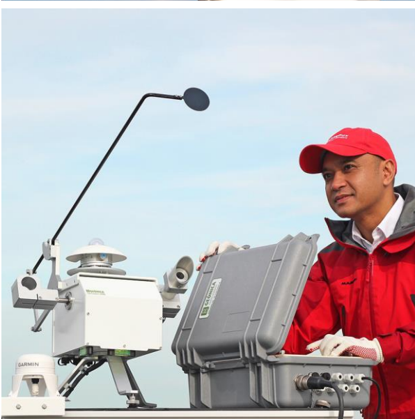
Figure 6 Pyrheliometers mounted on solar trackers
