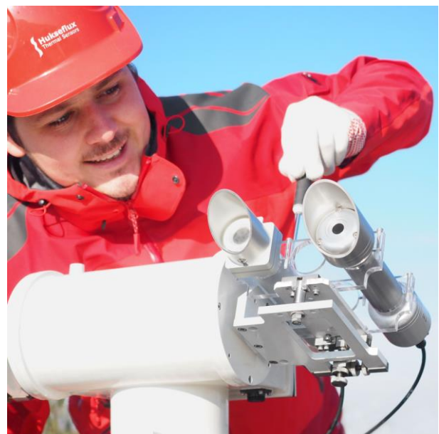
Figure 10 Pyrhelimeters with window heating (right) are effective to mitigate snow, frost and dew deposition on the window, providing the user with more valid data points.
