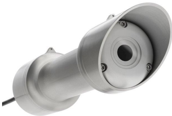
Figure 1 A pyrheliometer is pointed at the sun to measure the solar irradiance coming directly from the sun.
