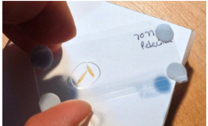
Figure 1. Bisected and bleached hind tibiae of Pelecinus polyturator in glycerin droplet between 1.5 thickness coverslips supported by Blu-Tack marbles.
