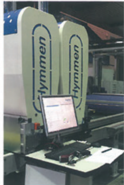
Figure 10: The JURITER Digital Printing Line for DLE here with two rows of printing heads at the Hymmen technology centre
