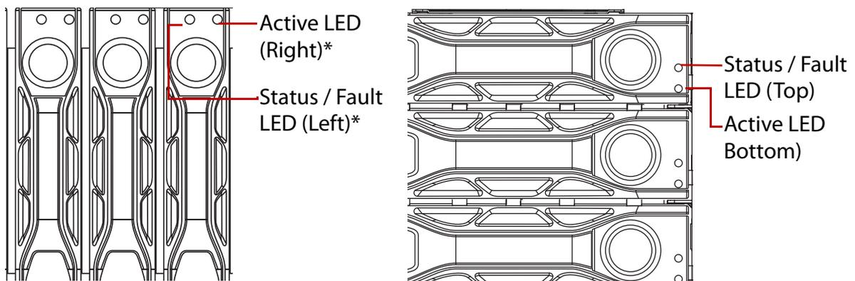
Figure 1-8. HDD LED Identification (\*only for QuantaGrid D51B-2U)
