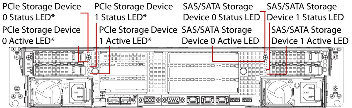
Figure 1-9. Rear Storage Device View (\*only for QuantaGrid D51B-2U)
