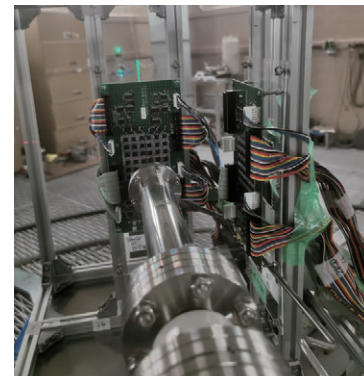
Experiment to evaluate the reliability of an integrated system against cosmic rays
