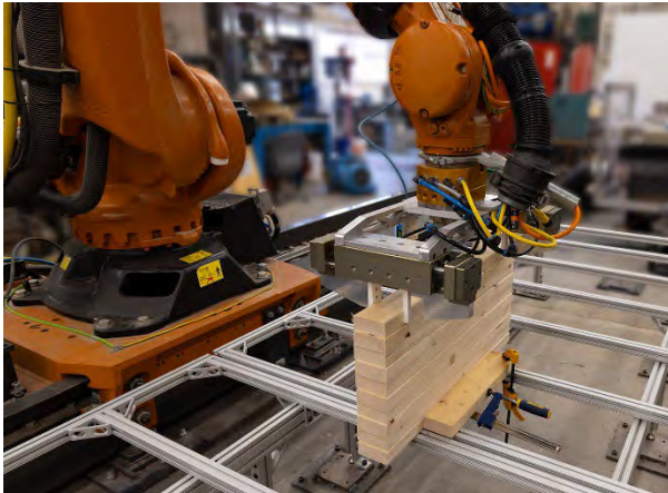
Figure 3. The South robot placing the final element in a timber stacking task (with no adaptation).
