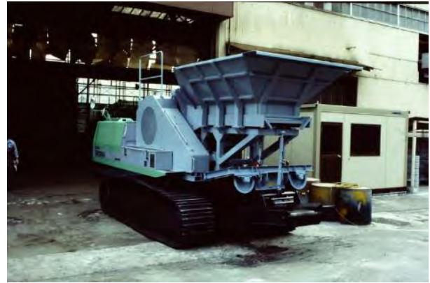
Figure 16. Concrete dismantling and concrete recycling robot Garapagos (Photo: T. Bock)
