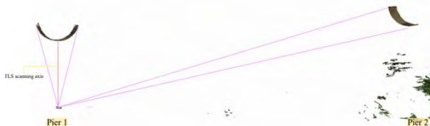
Figure 10: Scan coverage area while locating TLS perpendicular to the first pier
