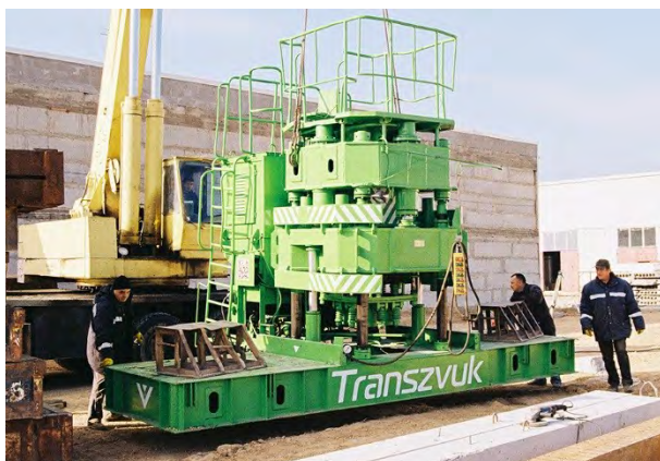
Figure 2. Piling Machine CO-450
