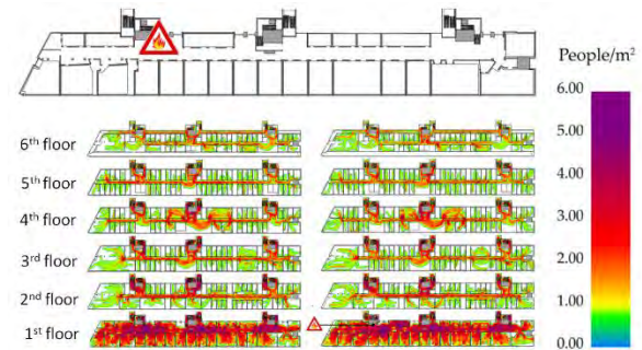
Figure 3. First floor with the hazardous event (Top side) and density maps from the first and second simulated scenario (Left and right bottom side respectively).
