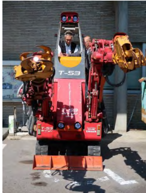
Figure 6. Maintenance robot Enryu T-53 developed by TMSUK Co. Ltd. (photo: T. Bock)
