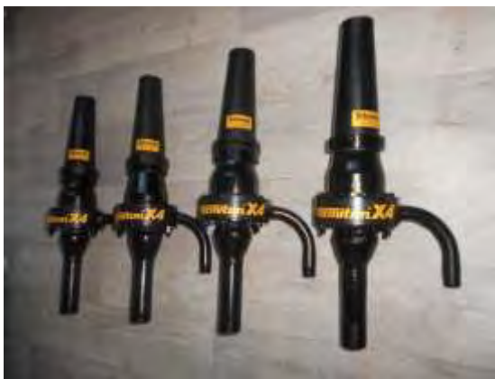
Figure 2. Shaft modification for semi-dry shotcrete
