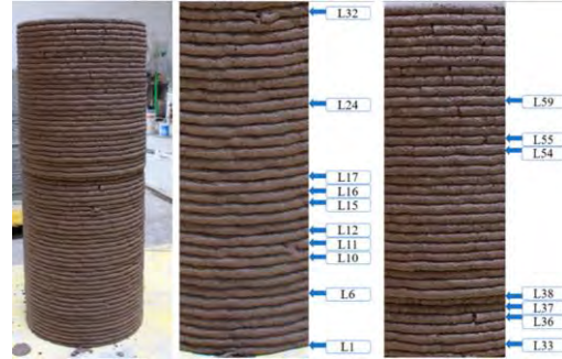
Figure 2 - Printed element A (left), bottom section of Element A taken for analysis - Section A1 (middle), Top section of Element B taken for analysis - Section A2 (right)
