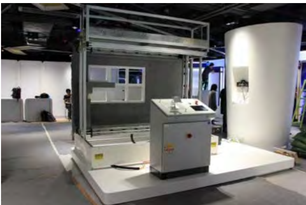
Figure 11. The semi-functional prototype of the multifunctional façade-processing robot exhibited in the Construction Innovation and Technology Application Centre in Hong Kong (photo: R. Hu)
