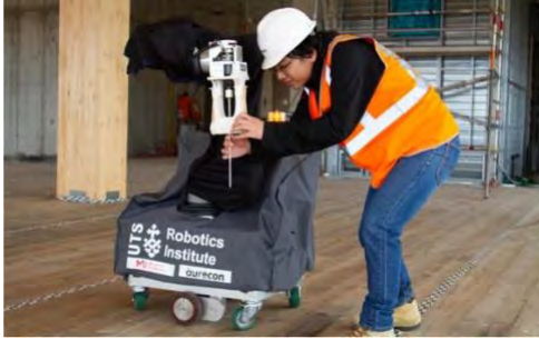
Figure 2. Intelligent robot prototype with human operator feeding screws
