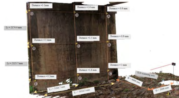
Figure 9 Measurement of point cloud spacing a_h , a_v along L_y & L_z
