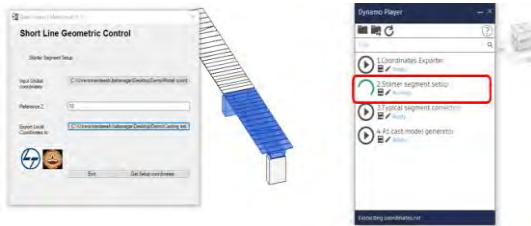
Figure 9: Starter segment setup module
