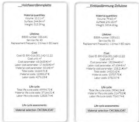
Figure 7. Example for material evaluation and material selection (left: Insulation Board, right: Cellulose Insulation)
