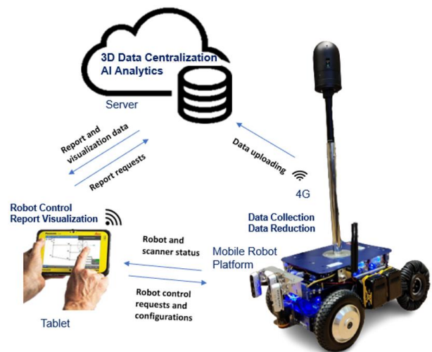
Figure 1. Overview of the System: It consists of (i) Mobile-robot platform, (ii) 3D and AI Analysis software on the cloud, (iii) Web-based user interface for robot control and defect
