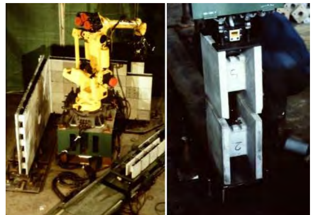
Figure 7. The SMAS robot developed for the assembly and disassembly of reinforced concrete blocks using ROD concept (photo: T. Bock)
