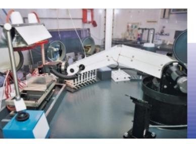
Zymark Robot for separation of U, Pu and fission products in spent fuel samples.
