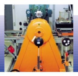
left: Cs-137 unit for radiation protection calibration right: Cobalt-60 unit for radiotherapy calibration. Both units are installed at the Dosimetry laboratory.
