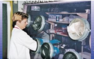
samples are handled in the glove box of the ICP/MS.
