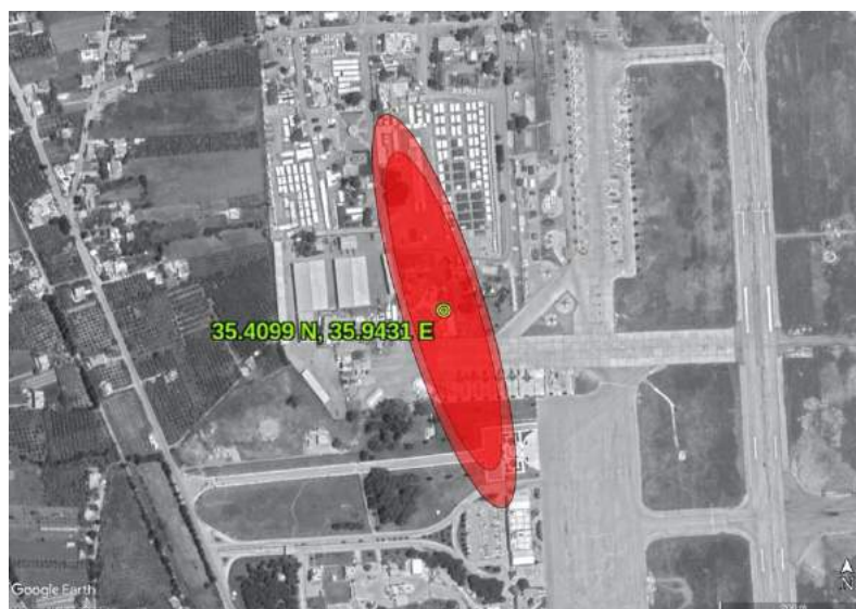
Figure 1. Estimated transmitter location overlaid on formal-error 95% and 99% horizontal error ellipses. The location is coincident with an airbase on the coast of Syria. The semi-major axis of the 95% ellipse is 220 meters.
