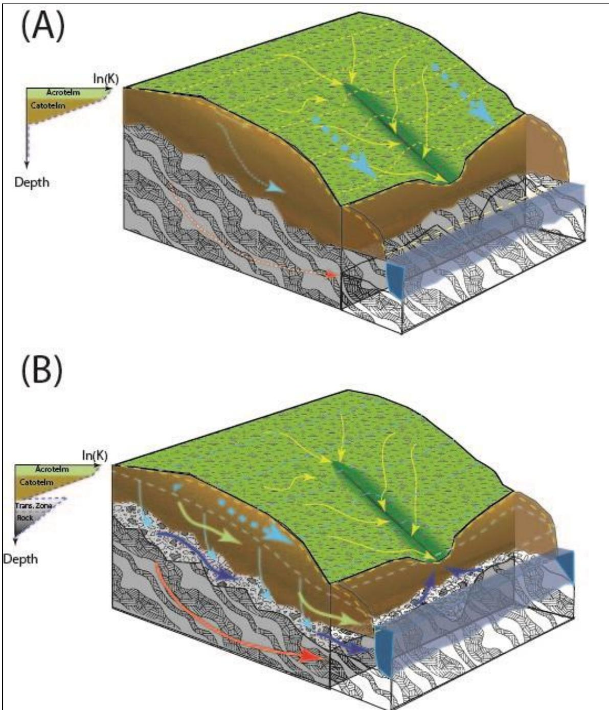
Figure 21: (Above) Conventional model of blanket bog hydrology with substrate contributions to stream flow proving negligible. (Below) Revised conceptual model, with significant substrate contributions.
