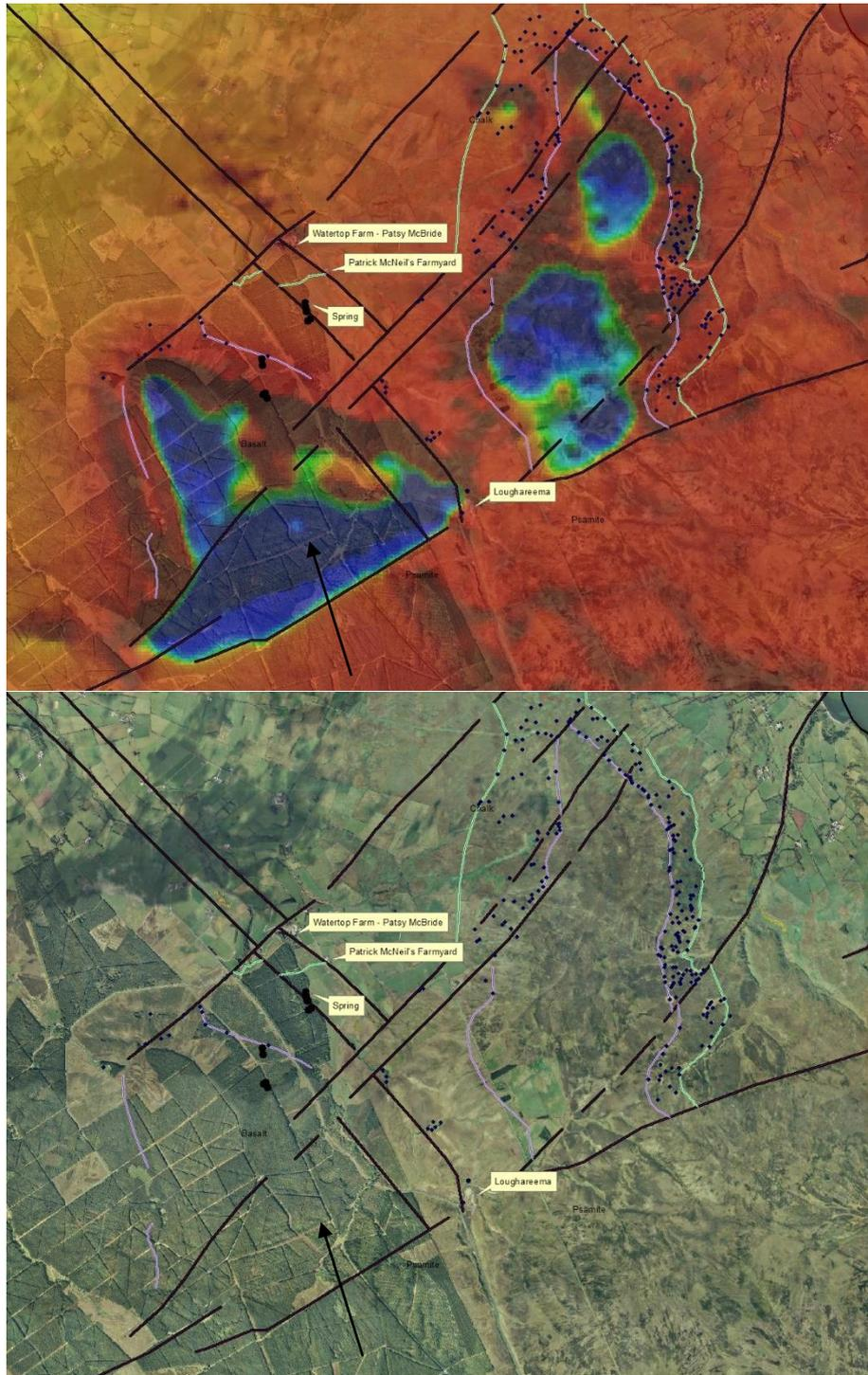
Figure 27A and B - Tellus Project magnetics with interpreted faults (black lines), base of Antrim Lava Group basalt (pink lines) and base of Ulster White Limestone Formation Chalk (green lines). Karstic features shown as points, and meltwater channel by black arrow.
