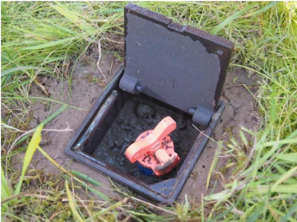
Figure 71: Completed Piezometer.
