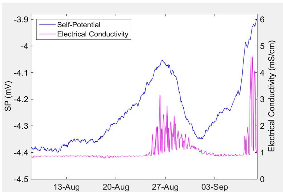
Figure 78: Spontaneous potential response in a chalk aquifer, occurring in advance of the intrusion of salt water. A significant time between the two parameter responses difference provides a basis for alerting of the danger of salt water contamination of drinking water supplies. (Figure: Prof. Adrian Butler, ICL)
