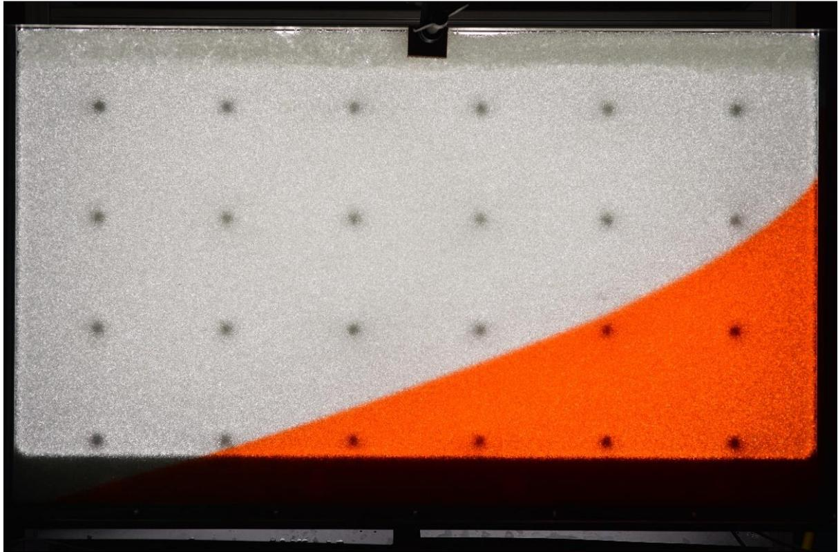
Figure 77: Image of laboratory apparatus employed to simulate salt water (red) intrusion into a saturated porous medium (glass beads) containing freshwater. The black points are ports employed to measure spontaneous potential while intrusion occurs. (Image: Georgios Etsias, QUB)
