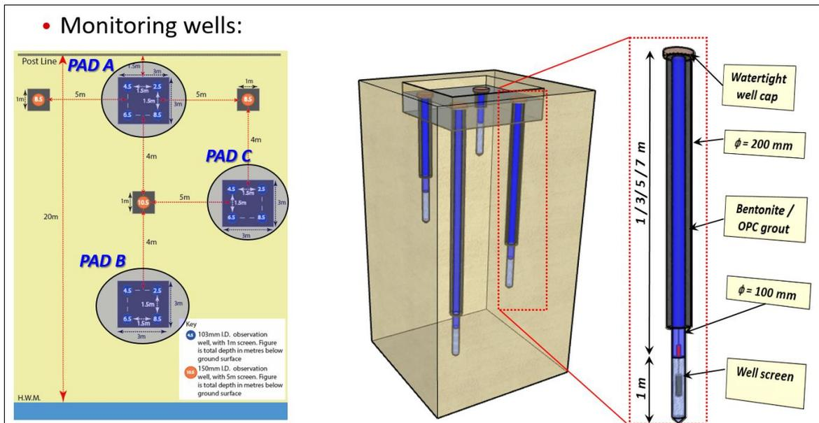
Figure 81: Observation well design for the Magilligan Test Site. Each pad has four 4" observation wells screened up to 8.5m below ground. All wells monitored water level temperature, electrical conductivity and spontaneous potential during pumping.
