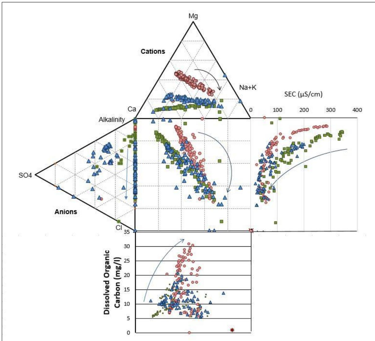
Figure 19: Expanded Durov plot summarising water quality in the streams draining the three test catchments. (Squares-Letterunshin, Circles-Garron, Triangles-Cuilcagh). Arrows reflect the evolution of water quality as flow increases, in which catchment waters with distinct base flow chemistries converge toward a common low SEC Na-Cl water type.
