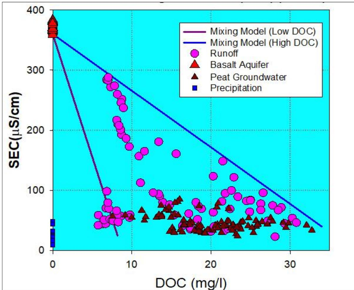
Figure 20: Plot of Specific electrical conductance with dissolved organic carbon content in end members and stream runoff for Garron Test Catchment. The lines reflect mixing models that view all runoff as derived from peat groundwater and from peat substrate, with inorganic substrate groundwater quality resembling that of the basalt aquifer. The model utilises high and low SEC and DOC contents in peat to span the ranges of variation observed in groundwater sampling.
