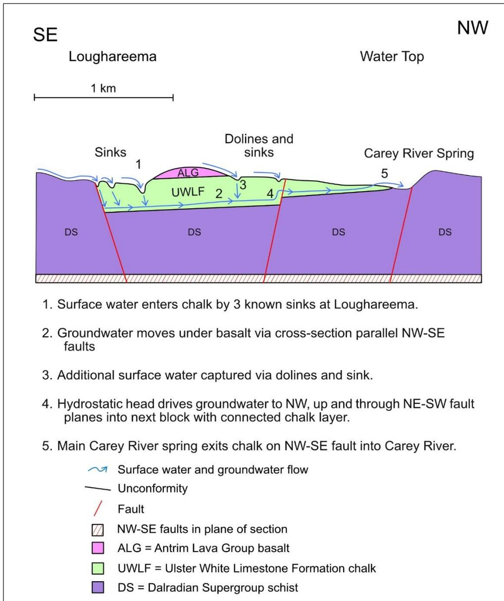
Figure 25: Schematic section through Loughareema and Carey Valley showing karstic features, surface and groundwater flow and relationships with faulting (no vertical scale).
