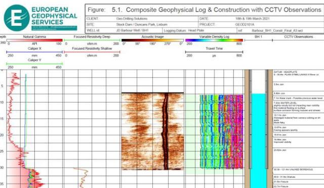
Figure 12: CCTV Survey & Cement (Sonic) Bond Log (VDL, TT). Mar-21.
