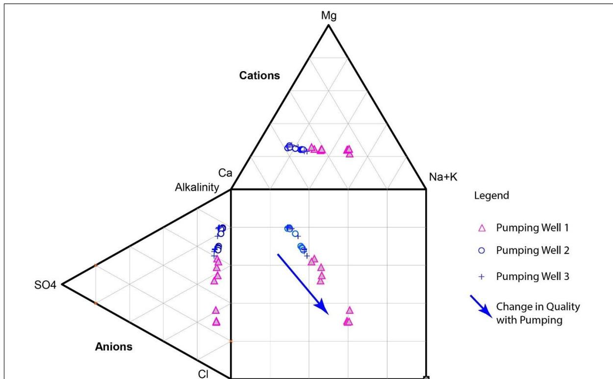
Figure 82: Durov plot illustrating changes in major ion content with pumping as additional saltwater was induced into pumping wells.
