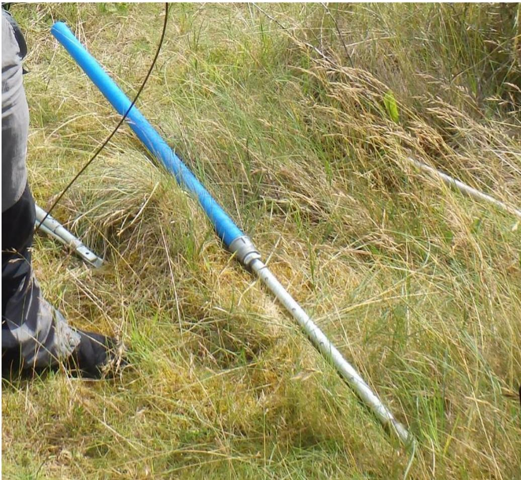
Figure 69: Hand installed Casagrande piezometer point.
