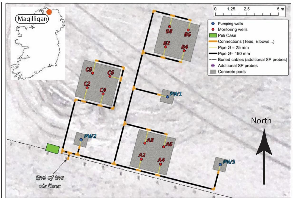
Figure 79: Location of Magilligan Test Site with positions of pumping and observation well clusters.
