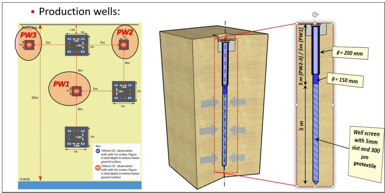
Figure 80: Pumping well design for the Magilligan Test Site. Wells PW2 and PW3 were pumped to intercept seaward-flowing fresh groundwater to enhance the possibility of drawing in salt water at PW-1. Well head water quality was measured with flow through cells at all three wells during pumping.
