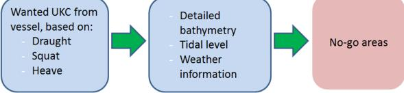
Figure 1: The diagram shows parameters needed to calculate the UKC advice. (Source: Porathe, 2006)
