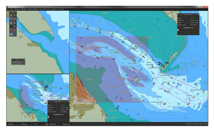
Figure 9: VTS operator may request No-Go for vessels in the area. Possible to have different No-Go depths contours shown in the different windows.
