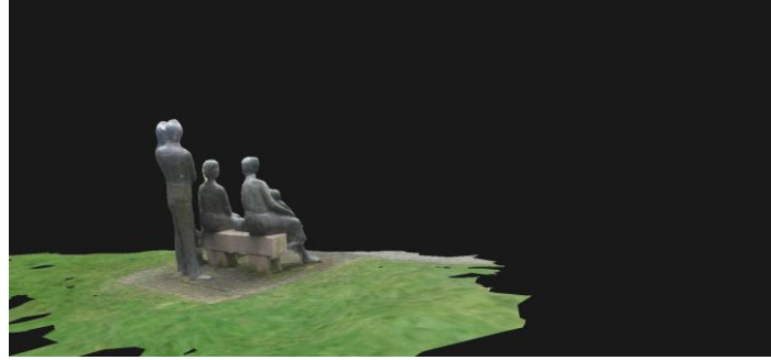
Figure 10. 3D object obtained from automated reconstruction from 176 images through NOC3D. Figure 8 shows exemplary images used in the reconstruction process for this 3D object. This is the default unmodified view, which appears offset. The black background is rendered by the 3D object viewer, in this case 3DEdit.
