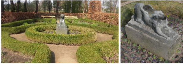
Figure 18. On the left: Statue “Panther” in a botanic garden in the Hanseatic City of Luebeck. On the Right: The output from 175 photos is hardly recognizable as a panther.
