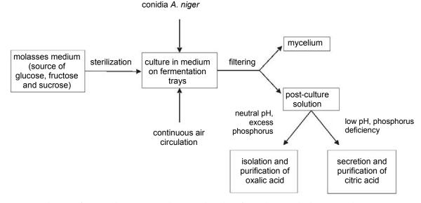
Figure 3. Production of citric acid using Aspergillus niger though surface culture method (Swain et al., 2011)
