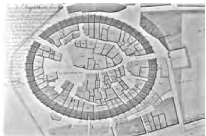
Figure 205. The Arena of Nîmes in 1809. Measured drawing by architect Grangent showing mediaeval houses still standing as well as those already demolished
