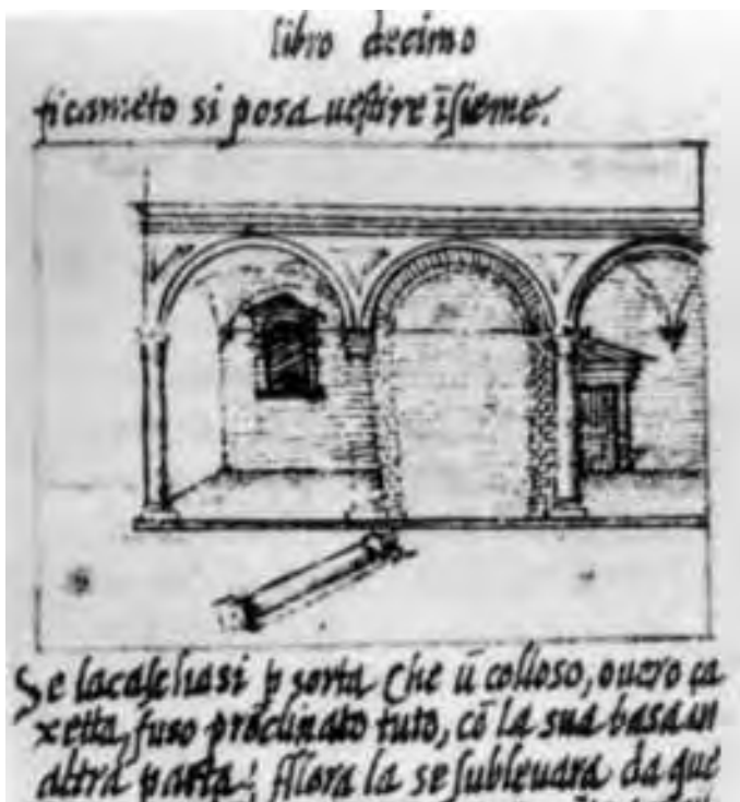
Figure 5, Illustration to Alberti's De re aedificatoria , showing his advice on replacement of damaged columns.
