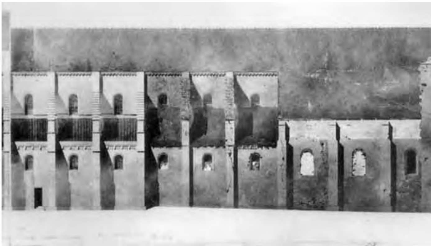
Figure 192. Viollet-le-Duc, La Madeleine, the north elevation before and after restoration (1840)
