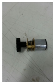
Figure 2. Morphing mechanism: (a) and (b) DC Motor and gear motor mounted to shaft
