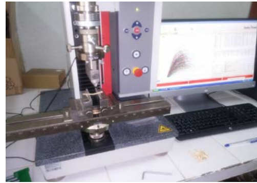
Figure 2. (a) Standard-size bending test sample and test setup (b) Micro-size bending test sample and test setup
