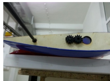
(c) Placement of the Servo motor in the wing
