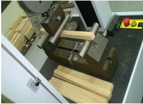
Figure 2. (a) Standard-size bending test sample and test setup (b) Micro-size bending test sample and test setup
