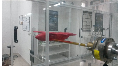
Figure 3. Wind Tunnel Test: (a) Spherically Blunted Tangent Ogive Nose
