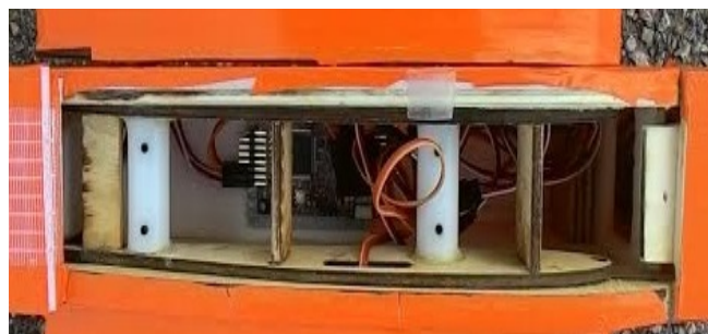
Figure 6. Autopilot Equipment of ZANKA-II
