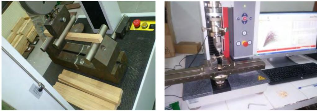
Figure 2. (a) Standard-size bending test sample and test setup (b) Micro-size bending test sample and test setup
