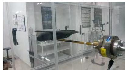
Figure 3. Wind Tunnel Test: (a) Spherically Blunted Tangent Ogive Nose
