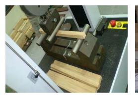
Figure 2. (a) Standard-size bending test sample and test setup
