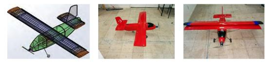
Figure 1. Aerial Robot: (a) Solidworks drawing of it
