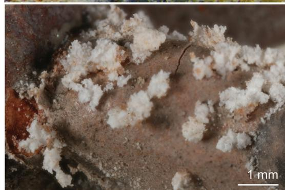
**Figure 3.** (top) Detail of the angel's wing showing flaking overpaint, white efflorescence, and rust-brown scales of chloride corrosion · Courtesy C. Hauer, ABK
