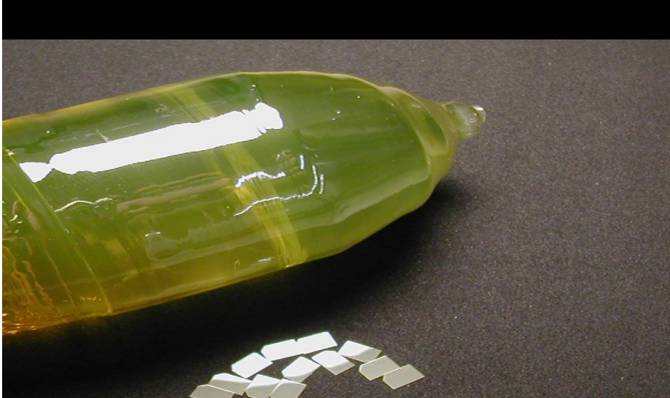
Fig. 1. \text{Al}_2\text{O}_3\text{:C-Mg} crystal and 4 \times 6 \times 0.5 \text{ mm}^3 FNTD (Akselrod et al., 2003).
