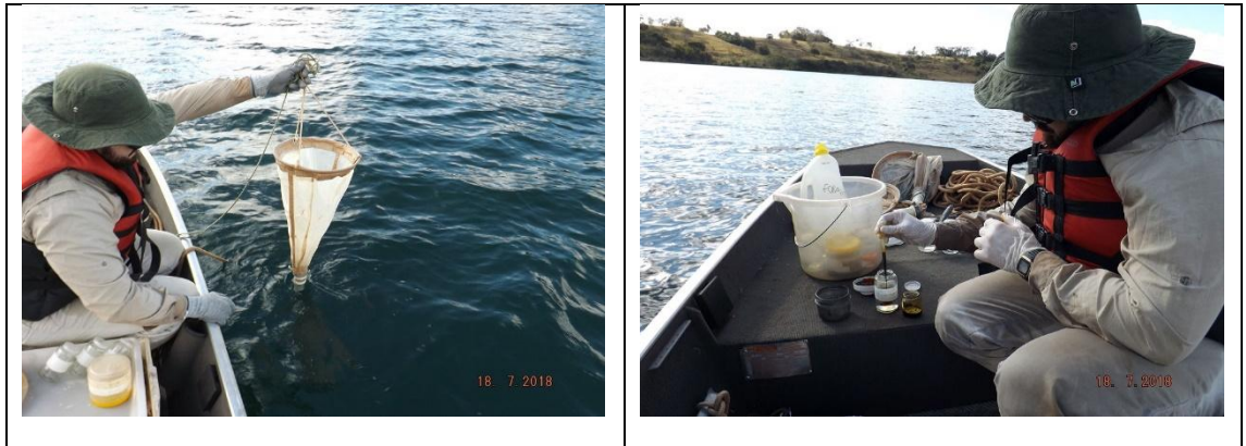
Figure 42 – Planktonic communities collection methodology at the Araguari River on July 2018 (collects with conical-cylindrical nets at the left and fixing of phytoplankton with lugol's iodine at right)
