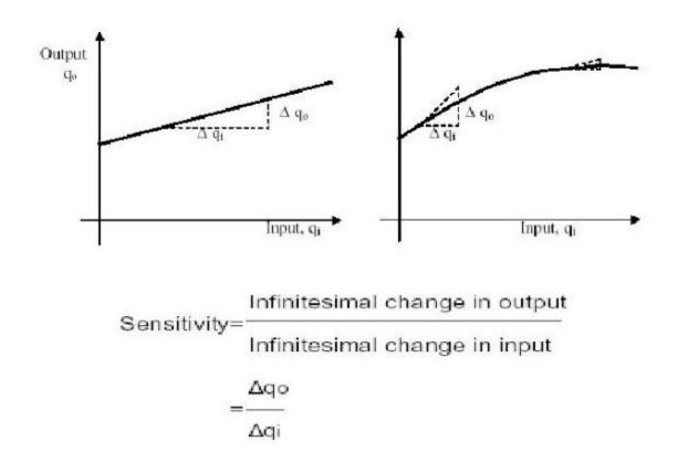
Thus, if the calibration curve is liner, as shown, the sensitivity of the instrument is the slope of the calibration curve. If the calibration curve is not linear as shown, then the sensitivity varies with the input. Inverse sensitivity or deflection factor is defined as the reciprocal of sensitivity. Inverse sensitivity or deflection factor = 1/ sensitivity
