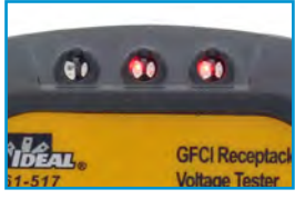
Red Lights Indicate Incorrect Wiring
