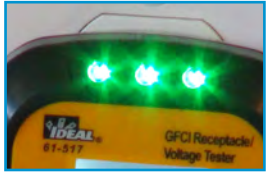
Green Lights Indicate Correct Wiring
