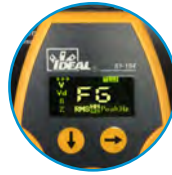
Detects and Displays false or "bootleg" ground
