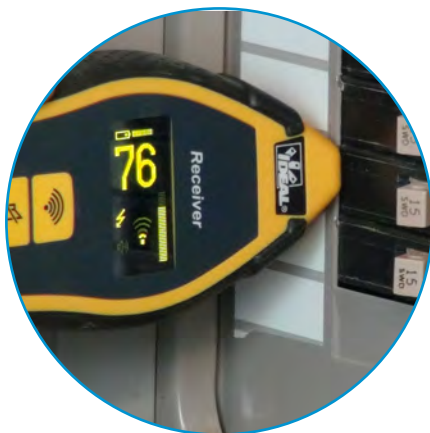
Finding Breakers or Fuses
