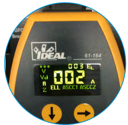
Estimated Load on Line in Amps
