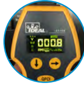
Displays neutral to ground voltage
