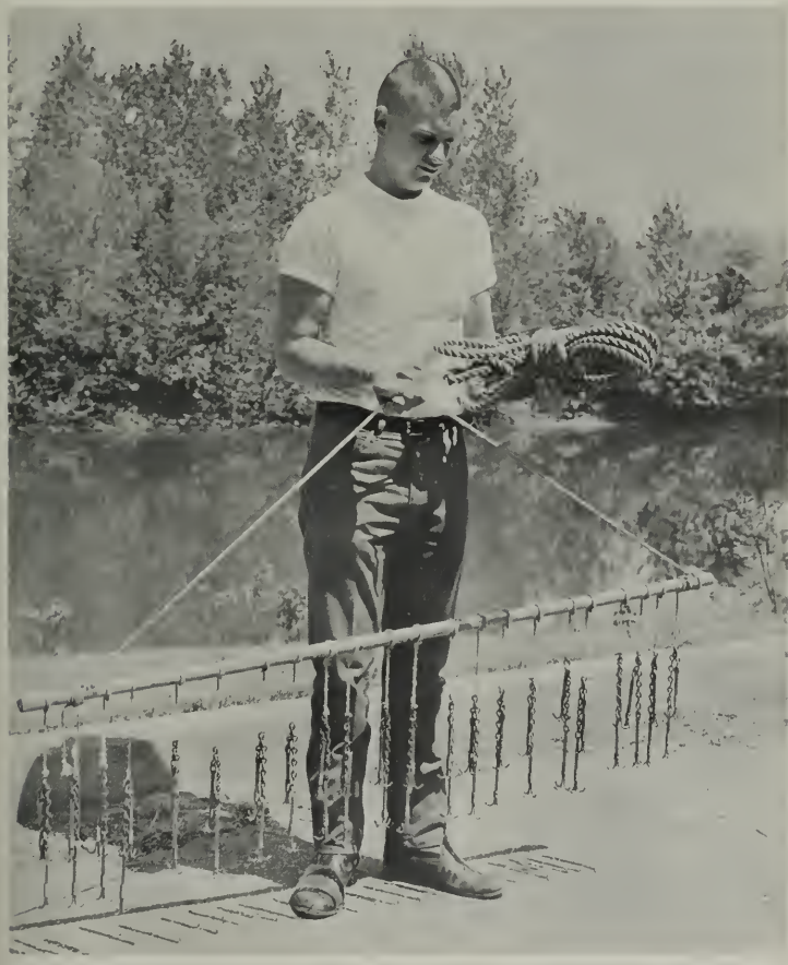
Fig. 5.—The exploratory crowfoot bar used on the Illinois River in the 1966 mussel survey. Photo by W. D. Zehr.
