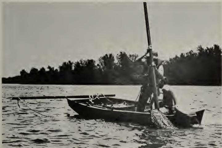
Fig. 8.—Lowering the dredge into the Illinois River during the 1966 mussel survey. Note the temporarily mounted boom on the bow of the boat to which the brail line was secured. From a color photo by the author.
