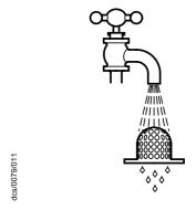
Figure 14 - Flush the filter
