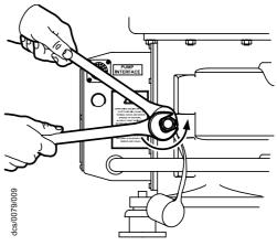
Figure 12 - Remove the filter inlet fitting
