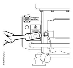
Figure 15 - Refit the filter
