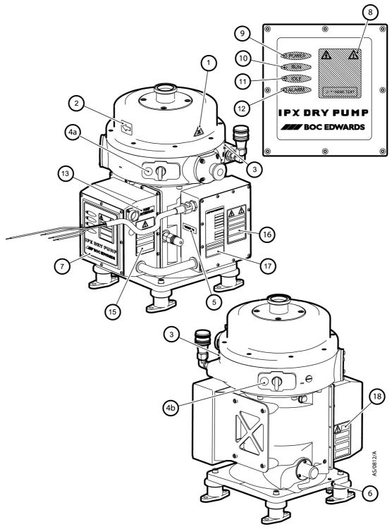
Figure 5 - Labels on the IPX A pump
