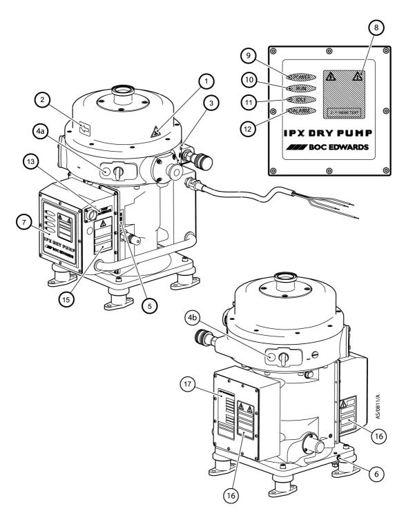
Figure 4 - Labels on the IPX pump
