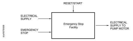
Figure 11 - Schematic diagram of emergency stop facility
