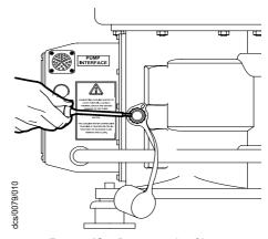
Figure 13 - Remove the filter
