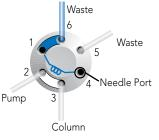
Flow path for the typical dual mode injector
