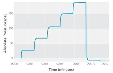
This graph shows the overlaid output from ten pressure sensors monitoring the same fluidic channel. High reproducibility and the capability for simultaneous reading of multiple sensors make the units extremely valuable for instrumentation applications. In this plot, the sensors are responding to a series of pressure increases over the sensor range.
