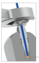
EXTRA INTERNAL VOLUME MarvelX UHPLC fittings do not depend on ferrules. They seal at the bottom of the port, without complex techniques, which significantly reduces required torque and enables many more connects and disconnects. Furthermore, they are virtually impossible to over-tighten by hand, limiting wear and increasing product life. An enhanced proprietary tip design also ensures zero dead volume (ZDV) and better chromatography results.
