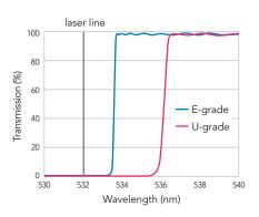
The spectral response of a U-grade filter is located anywhere between the red and blue lines below.
