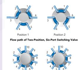
Flow path of Two-Position, Ten-Port Switching Valve
