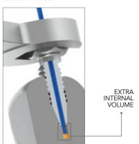
MarvelXACT fittings do not depend on ferrules. They seal at the bottom of the port, without complex techniques, which significantly reduces required torque and enables many more connects and disconnects. MarvelXACT significantly reduces wear on your hardware, increasing product life. An enhanced proprietary tip design also ensures zero dead volume (ZDV) and better chromatography results.
