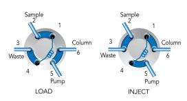
Flow path of Two-Position, Six-Port Injection Valve
