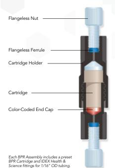
Choose from our line of Biocompatible and Stainless Steel BPR Assemblies, each complete with a replaceable, factory preset cartridge (except the 5 and 20 psi versions).
