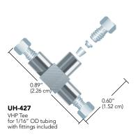
Our VHP Stainless Steel Tees and Crosses are precision machined from durable stainless steel. It is mechanically designed for bringing together three or four pieces of tubing. Our VHP Tees & Crosses have an extremely high pressure rating of 30,000 psi (2070 bar).
