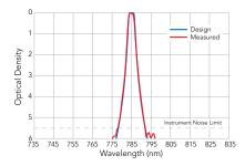
These graphs demonstrate the outstanding performance of the 785 nm MaxLine laser-line filter, which has transmission guaranteed to exceed 90% at the laser line and 0D > 5 blocking less than 1% away from the laser line. Note the excellent agreement with the design curves.
