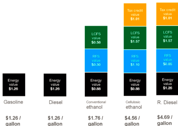
Figure 2.20. Average market value of cellulosic ethanol and renewable diesel compared to other fuels in California in 2019 (Lane, 2020)
